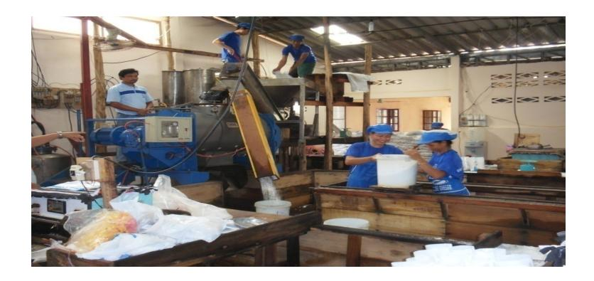
batch production with a paddle mixer good results for a combined mixture of KIO<sub>3</sub> and KF, perfectly homogeneous
